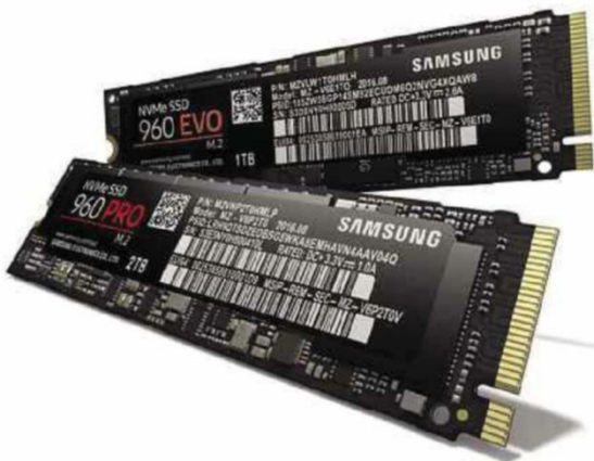
▲ M.2 NVMe storage. The size of a stick of gum and six times the speed of the very best SATA SSD
